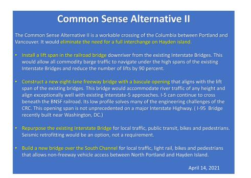
The Common Sense Alternative II is a workable crossing of the Columbia River between Portland and Vancouver. It would eliminate the need for a full interchange on Hayden Island and be over a billion dollars less expensive than the formerly approved "locally preferred alternative".
