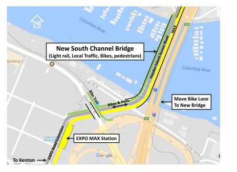
This diagram shows the new South Channel Bridge in even more detail. The yellow line shows the MAX route, the gray line shows the auto and truck route and the green line shows a bike path, including access to the Marine Drive bicycle path.
