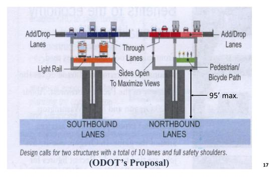
This ODOT slide illustrates a cross section of the "Locally Preferred Alternative" new 10-lane I-5 bridge far above the river, mixing local traffic with interstate traffic. There is no alternative route available here, should there be a serious traffic issue on the interstate.
